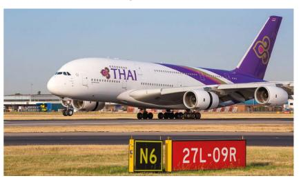
The example above indicates that your location is N6, holding short of Runway 27L/09R. The Runway 27L threshold is to your left, and the 09R threshold to your right.
