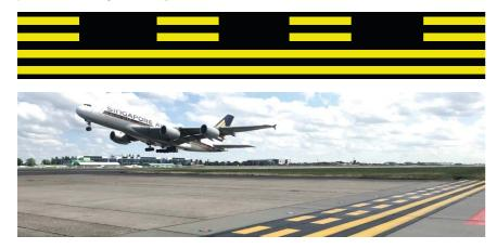
At Heathrow this will either indicate a CAT I holding point, or a combined CAT I and CAT II/III holding point (when there is only one runway holding point).
