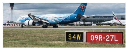
The example above indicates that you are at location S4W, holding short of Runway 09R/27L. The Runway 09R threshold is to your left; the Runway 27L threshold is to your right.
