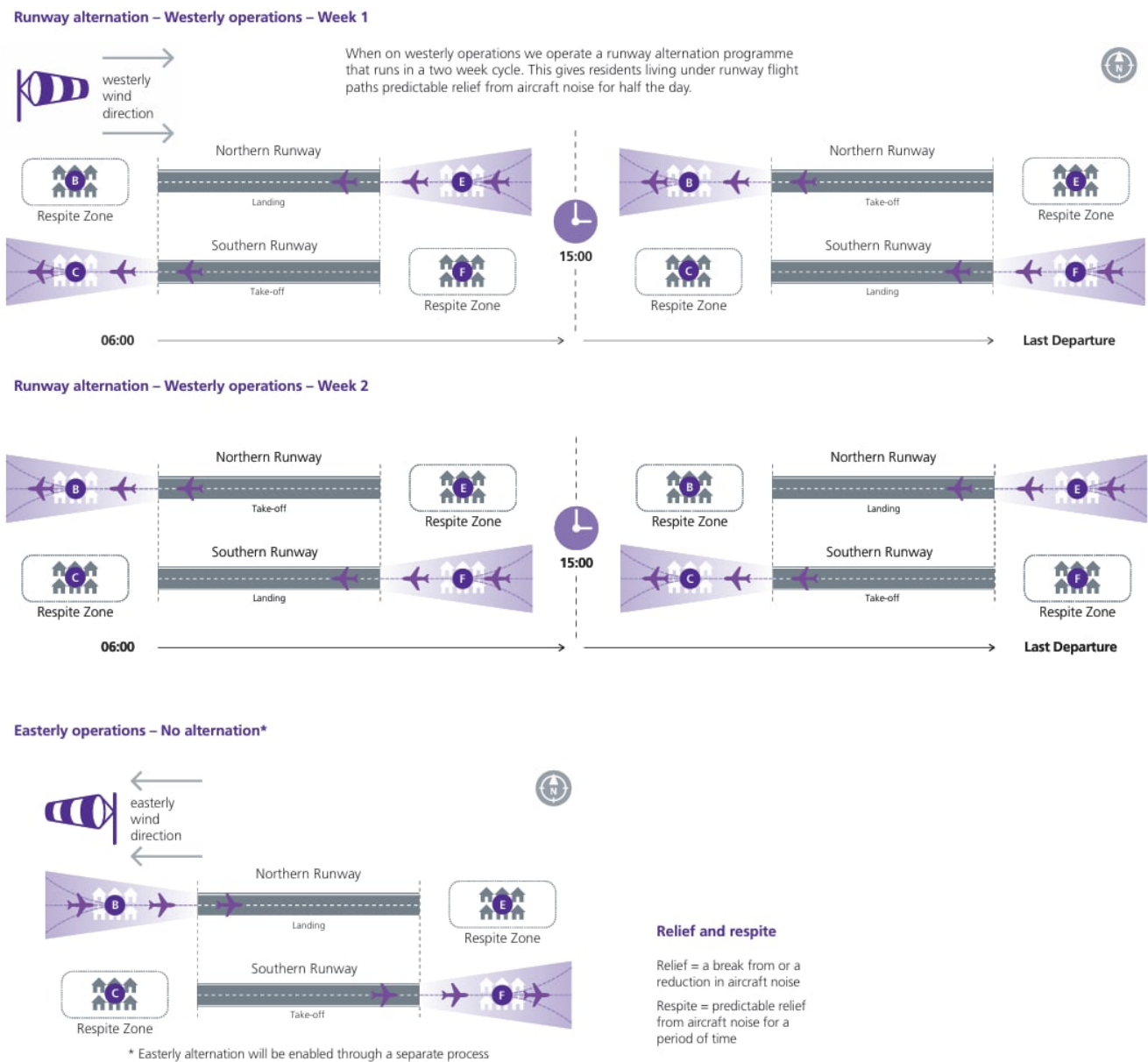
Figure 2.3: Current runway alternation (westerly and easterly operations)
